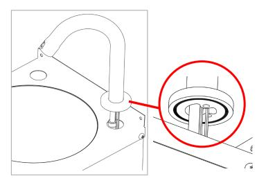
5.3 Install the tap fixing kit from beneath the basin. Tighten the nuts using a 9mm spanner. **IMPORTANT:** Do not overtighten.
