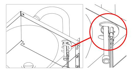
5.4 Connect the microvalve to the hose coming out of the tap. **IMPORTANT:** Do not overtighten.
