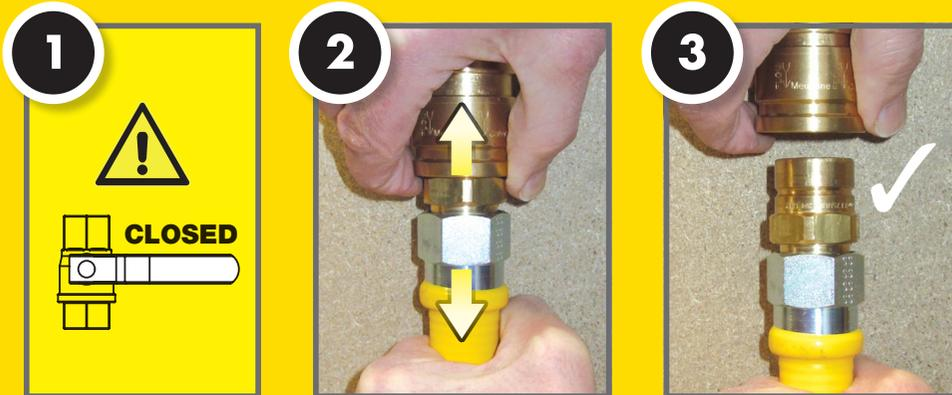
Firstly isolate the gas supply by turning the local isolation valve to the 'closed' position. Grip the outer collar of the QD coupling and, whilst holding the hose, pull back the collar to release the inserted male part.
