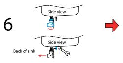
Tighten buffer against underside of bowl Lock in place.
