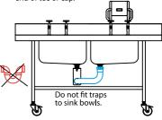
Water / drain connections
