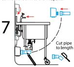
Offer drain fitting against wall. Mark cut length - allow for socket.
