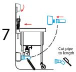
Offer drain fitting against wall, Mark cut length - allow for socket.
