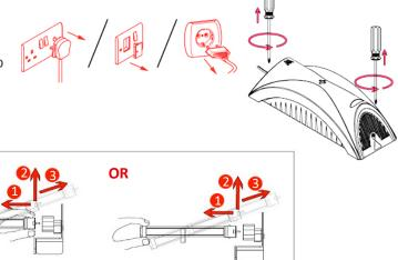
If you are fitting a NEW lamp, firmly grip lamp terminal/connector end (or end cap) and carefully slide lamp into the socket and spring clip.
