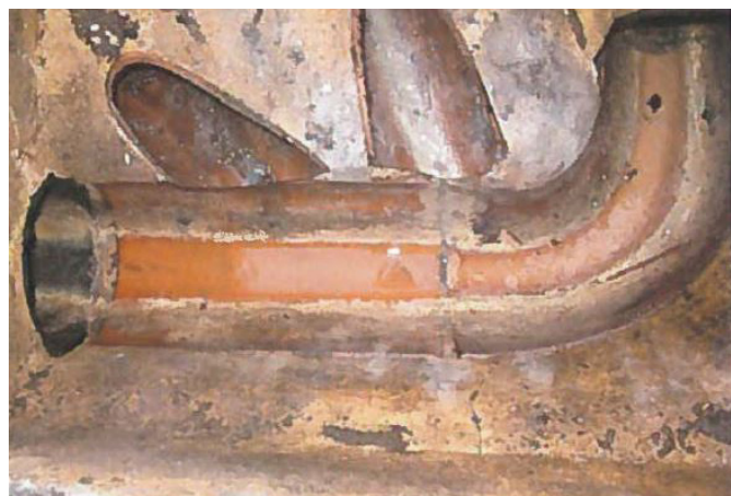
The clear sewer run at the end of the year-long trial, April 2017.
