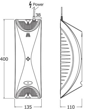
Dimensions are in millimeters. If a Cad file is required please visit <u>www.mechline.com</u>.
