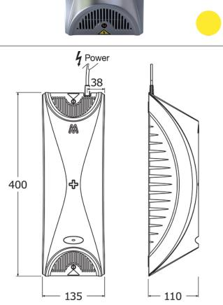
Dimensions are in millimeters. If a Cad file is required please visit <u>www.mechline.com</u>.
