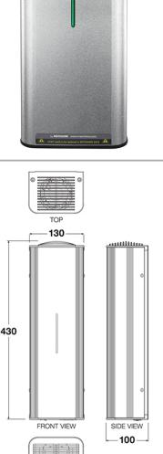
Dimensions are in millimeters. If a Cad file is required please visit  $\underline{www.mechline.com}.$
