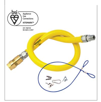
Dormont UNBRAIDED ½-inch 1000mm Gas Hose "NPVF" + Quick-Disconnect Coupling + Straight Restrainer Cable with mounting hardware
