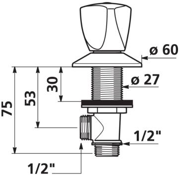
Dimensions are in millimeters. If a Cad file is required please visit  $\underline{www.mechline.com}.$
