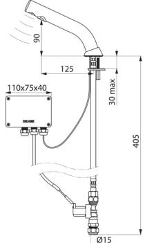
Dimensions are in millimeters. If a Cad file is required please visit <a href="www.mechline.com">www.mechline.com</a>.
