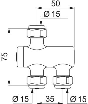
Dimensions are in millimeters. If a Cad file is required please visit  $\underline{www.mechline.com}.$
