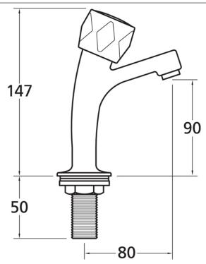
Dimensions are in millimeters. If a Cad file is required please visit <u>www.mechline.com</u>.
