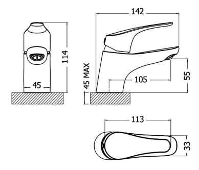
Dimensions are in millimeters. If a Cad file is required please visit <u>www.mechline.com</u>.
