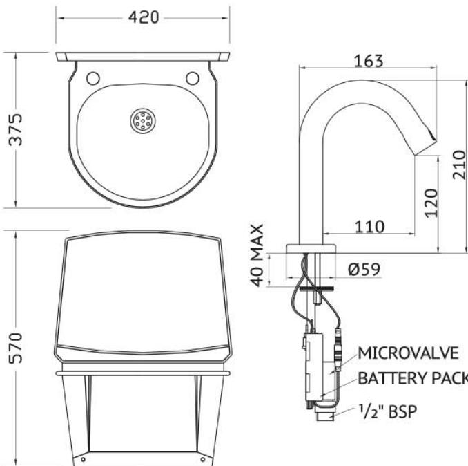
Dimensions are in millimeters. If a Cad file is required please visit [www.mechline.com](http://www.mechline.com).
