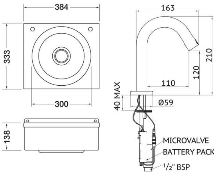
Dimensions are in millimeters. If a Cad file is required please visit [www.mechline.com](http://www.mechline.com).
