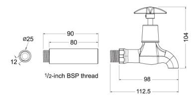
Dimensions are in millimeters. If a Cad file is required please visit <u>www.mechline.com</u>.
