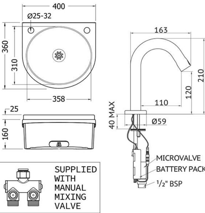
Dimensions are in millimeters. If a Cad file is required please visit [www.mechline.com](http://www.mechline.com).
