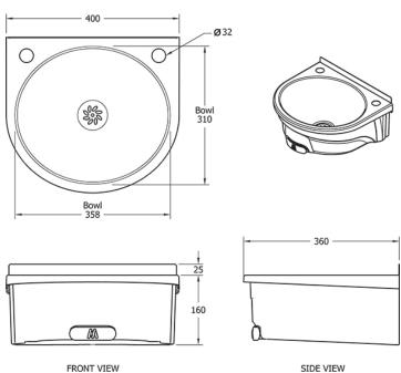
Dimensions are in millimeters. If a Cad file is required please visit <u>www.mechline.com</u>.
