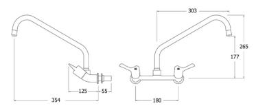
Dimensions are in millimeters. If a Cad file is required please visit <u>www.mechline.com</u>.
