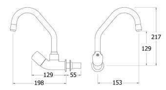
Dimensions are in millimeters. If a Cad file is required please visit <u>www.mechline.com</u>.
