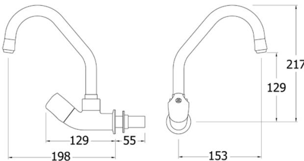
Dimensions are in millimeters. If a Cad file is required please visit [www.mechline.com](http://www.mechline.com).
