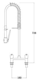
Dimensions are in millimeters. If a Cad file is required please visit <u>www.mechline.com</u>.
