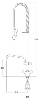
Dimensions are in millimeters. If a Cad file is required please visit <u>www.mechline.com</u>.
