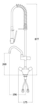
Dimensions are in millimeters. If a Cad file is required please visit <u>www.mechline.com</u>.
