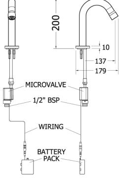
Dimensions are in millimeters. If a Cad file is required please visit <u>www.mechline.com</u>.
