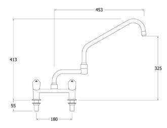
Dimensions are in millimeters. If a Cad file is required please visit <u>www.mechline.com</u>.
