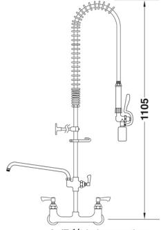
2x (F) 1/2-inch connections Tap hole req.: 2x 25mm dia.
