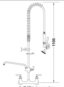
2x (F) 1/2-inch connections Tap hole req.: 2x 25mm dia.
