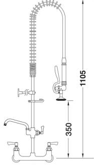
2x (F) 1/2-inch connections Tap hole req.: 2x 25mm dia.
