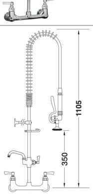
2x (F) 1/2-inch connections Tap hole req.: 2x 25mm dia.
