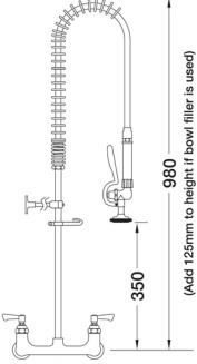
2x (F) 1/2-inch connections Tap hole req.: 2x 25mm dia.
