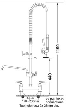
Dimensions are in millimeters. If a Cad file is required please visit <u>www.mechline.com</u>.
