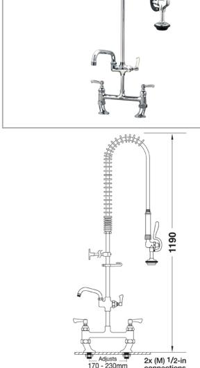
Tap hole req.: 2x 25mm dia. Dimensions are in millimeters. If a Cad file is required please visit www.mechline.com.
