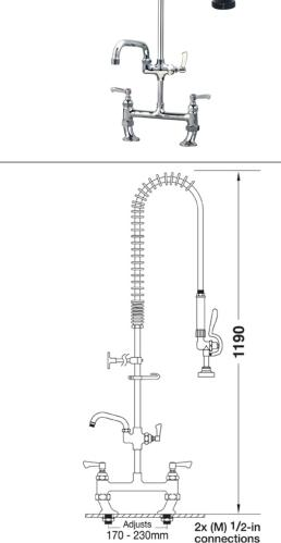
Tap hole req.: 2x 25mm dia. Dimensions are in millimeters. If a Cad file is required please visit www.mechline.com.
