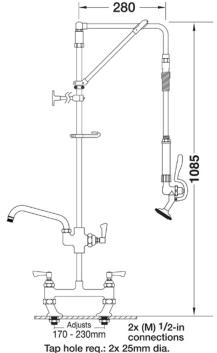
Dimensions are in millimeters. If a Cad file is required please visit <u>www.mechline.com</u>.
