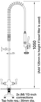
Dimensions are in millimeters. If a Cad file is required please visit <u>www.mechline.com</u>.
