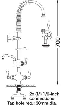
Dimensions are in millimeters. If a Cad file is required please visit <u>www.mechline.com</u>.
