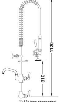
(F) <sup>1</sup>/2-inch connection Tap hole req.: 25mm dia.
