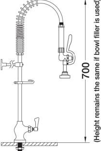
(M) 1/2-inch connection Tap hole req.: 25mm dia.
