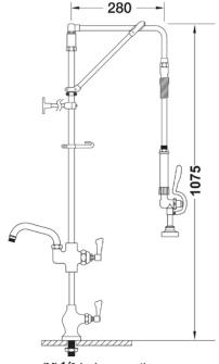
(M) 1/2-inch connection Tap hole req.: 25mm dia.
